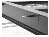
Fig. 1-Through Frame Crank Extension w/pin.
